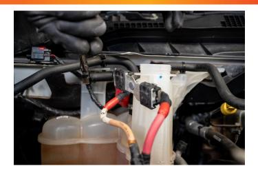
**STEP 11:** Locate the hose routed from the top of the coolant riser pipe. Remove the hose clamp from the fitting and disconnect the hose from the coolant riser shown at right.
