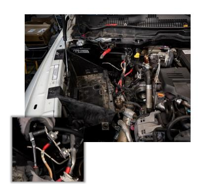
**STEP 24:** Reinstall the harness fir trees onto the battery tray and connect the wires to the solenoid using a 12mm socket or wrench.
