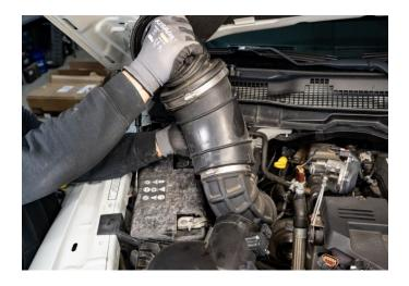
**STEP 5:** Remove the one bolt retaining the airbox assembly to the passenger side fender using a 13mm socket or wrench. Disconnect the active air connector on the lower driver's side of the airbox. Remove the airbox from the vehicle and set aside.
