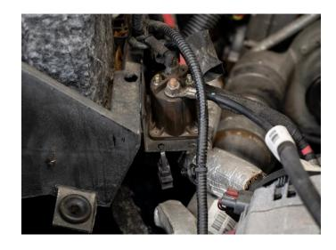
**STEP 8:** Using a 10mm socket or wrench, remove the bolt retaining the battery hold down clamp. Remove the passenger side battery. Using a trim tool, remove the fir trees retaining the solenoid harness to the battery tray.
