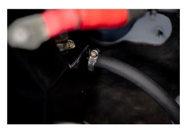
**STEP 21:** Install the included coolant overflow hose (12" cut length) onto the Fleece Performance coolant tank. Route the hose into the fender as shown at right.
