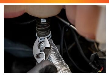
**STEP 14:** Disconnect the coolant level sensor on the underside of the OE coolant tank.
