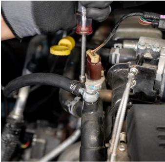
Place another hose clamp (SAE size 8) onto the other end of the hose and install the hose onto the driver's side facing hose barb on the Fleece Performance coolant tank. Tighten the hose clamp.
