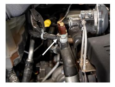
**STEP 12:** Locate the coolant de-gas hose on the top side of the OE coolant tank shown at right. Remove the hose clamp by prying the retainer away from the clamp. Disconnect the hose from the coolant tank.
