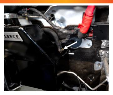
**STEP 20:** Place a hose clamp (SAE size 8) on one end of the included 3/8" hose (24" cut length) and install the hose onto the barb on top of the coolant riser pipe. Tighten the hose clamp.
