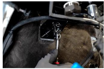
**STEP 19:** Place one of the included SAE size 8 hose clamps onto the OE coolant de-gas line and install the line onto the upward facing hose barb on the Fleece Performance coolant tank. Tighten the hose clamp.
