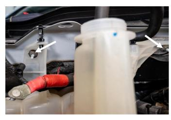
Once all three nuts are removed, remove the OE coolant tank.
