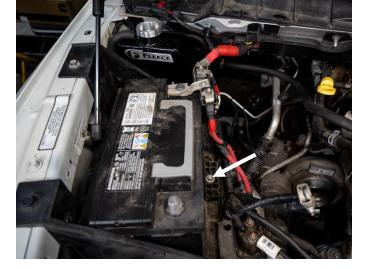
**STEP 27:** Connect the active air connector to the lower driver's side of the airbox and install the airbox into the vehicle. Using a 13mm socket or wrench, install the airbox retaining bolt. Connect the MAF and barometric pressure sensors.
