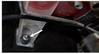
**STEP 16:** Using the included thread sealant, place a thin layer on the threads of the barbed NPT fitting. Install the fitting into the overflow port on the new Fleece Performance coolant tank using an 11mm socket or wrench.
