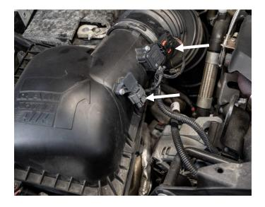
**STEP 4:** Loosen the hose clamp retaining the crankcase ventilation (CCV) tube to the intake tube. Disconnect the CCV tube. Remove the intake tube from the vehicle and set aside.
