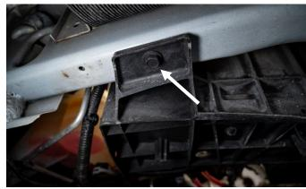
**STEP 10 (optional):** Using a 12mm socket or wrench, remove the nut connecting the main power cable to the battery bus bar. Set the bus bar and harness aside.
